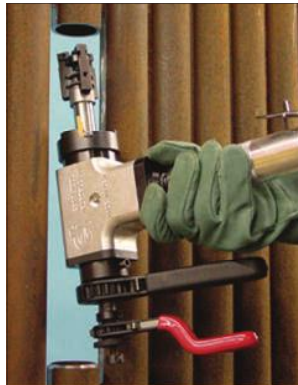
The "Tube Weasel" fits a Dutchman window for single tube end prep work and totally sealed construction allows it to be used in any orientation. Most importantly, the holding clamps are designed to stay on the mandrel and not fall down the tubes.
